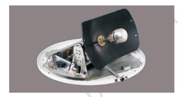
Probecom Land Mobile Communication Parabolic Antenna uses ring focus back feed antenna, it has high gain, the mobility is strong and tracking effect is superior. It is suitable for different kinds of communication.
