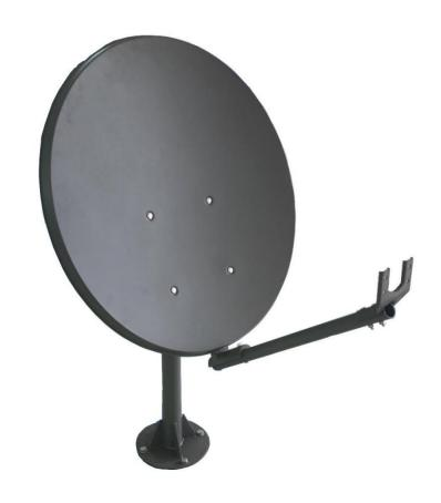
Probecom's Ka band offset VSAT series antennas adopt advanced surface treatment technology, which makes the antennas have the advantages of corrosion resistance and long lifetime. The antennas' surface accuracy (R.M.S) is less than 0.3mm and support various Ka transceivers in the market. Probecom's Ka band offset VSAT antennas are cost-effective and suitable for a wide range of applications. Products' size ranges from 0.74m, 0.98m and 1.2m.
